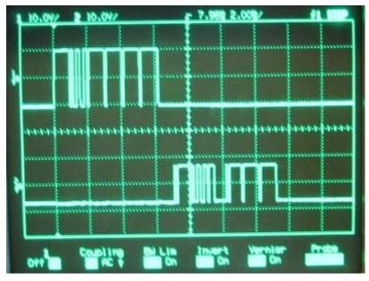
This is a closeup of the instruction bytes. Note that the voltage swing of the instruction waveform is about +/-10V. This is typical of the USB to RS232 converter to which the device is connected. The instruction bytes are 0, 51, 0, 0, 0, 0 indicating the instruction: Device: All, Command: Return version, Data: 0.
