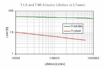
Note that the failure mode of T-LA devices is grease contamination by wear particles which effectively clog the lead-nut, although the lead screw and lead-nut remain in healthy condition. Extending the lead screw, cleaning it, and regreasing it with a silicon based grease effectively solves the problem; however, this may not be feasible in all applications. For more detailed
